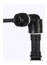
To run the 1/4" tubing parallel to the ground rather than straight up off of the riser, use a <u>Marlex Elbow</u>. This allows the tubing to run flat on the ground and avoids a trip hazard.
